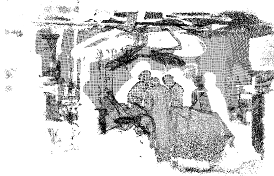
Figure 5: A visualization of the point cloud dataset from a point of view similar to the location of the Kinect that scanned the image.
